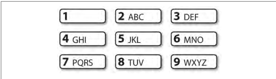
Figure 3-5. T9: Text on 9 keys.
